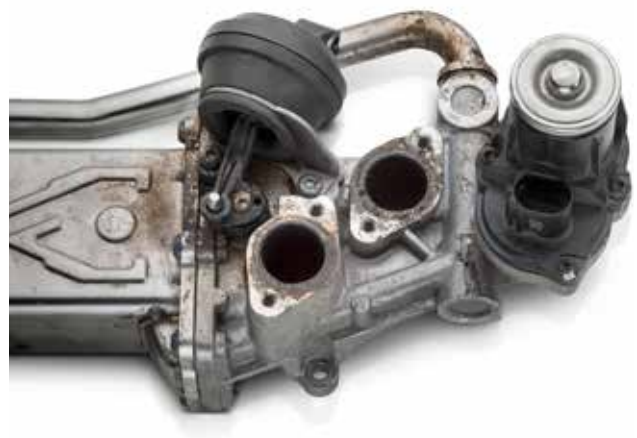
EGR cooler with servomotor and vacuum actuator
