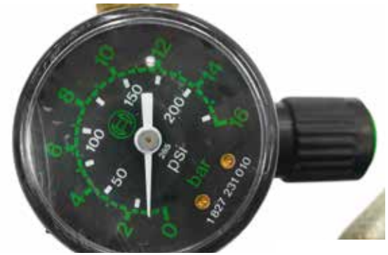
Manometer for pressure testing
