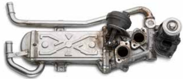
Removed EGR cooler
